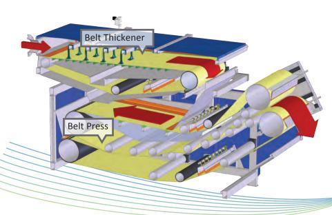
DEWA N-PD XL belt filter press is the most flexible solution for any type of sludge dewatering applications. N-PD "combo" belt filter press is combination of belt thickener and belt press. Drive units for both functions are equipped with combined frequency speed inverter. Both functions have individual pneumatic steering and tensioning systems. Spray cleaning for each belt separately can be done by standard nozzle pipes or with brush pipes.
